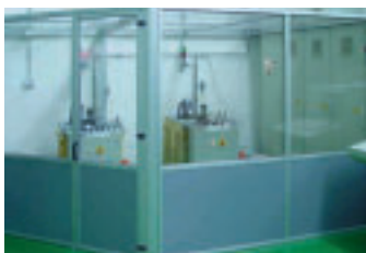
Test rig for alternator bearings: The rig uses inverters to control the motors and boost efficiency and is enclosed to reduce noise pollution.
